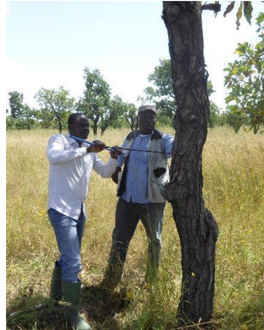
Picture 3. 2 Techniques of extraction of wood sample using increment borer. (CHABI, 2014)
