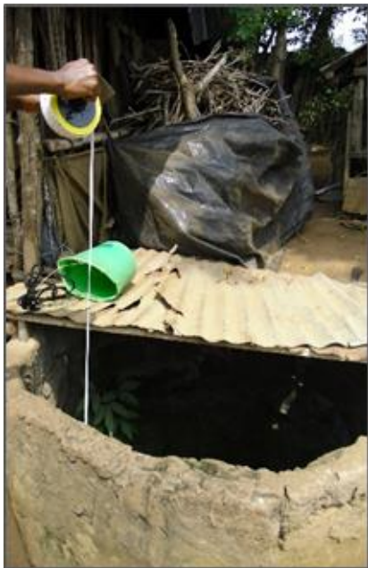
Photo 4: Measuring water level in a dug well in Songon-Té using water level meter (left) and a typical borehole in Nguessandan (right).
