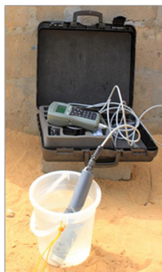
Photo 5: Some field measuring instruments. Handheld WAGTECH turbidity meter (left) and HANNA HI-9878 multiparameter hand held meter (right).
