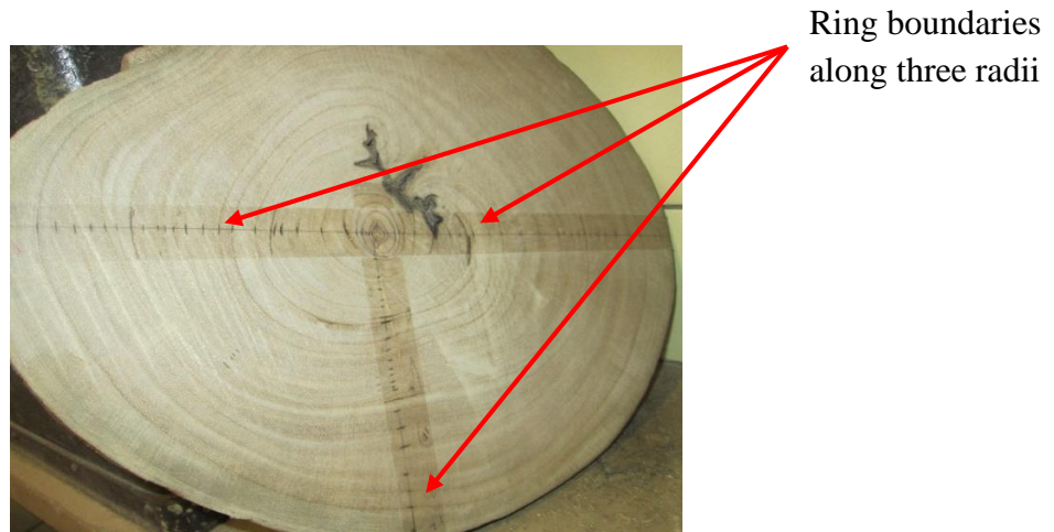
Photo 4: Stem disc with tree-ring boundaries marked along three radii
