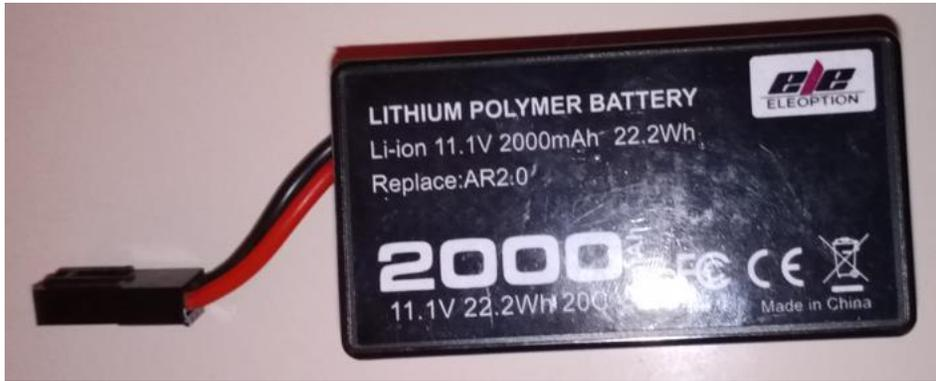
Figure 29: Lithium battery to power the smart WSD system.
