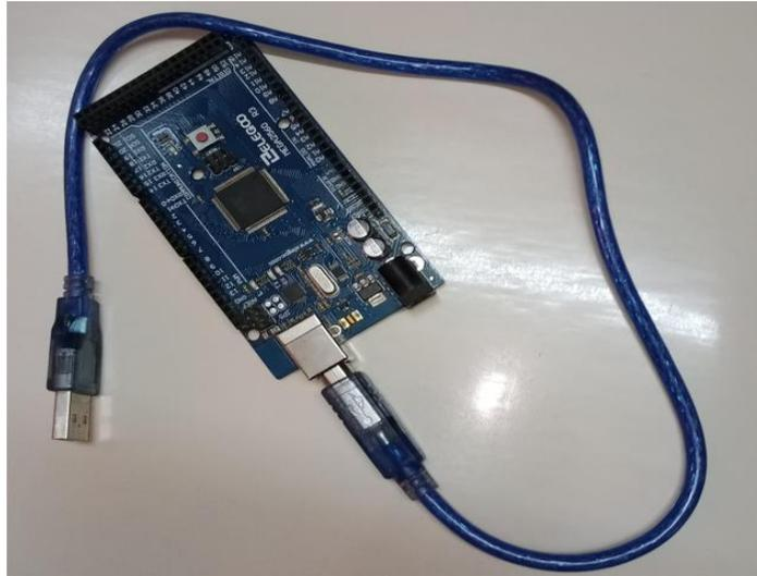
Figure 15: Arduino Mega 2560 Microcontroller.
