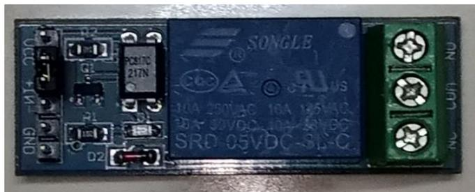
Figure 19: Relay Module.
