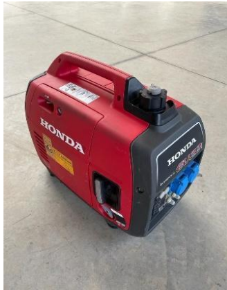
Figure 20: Generator use to power the okptopus inspection system
