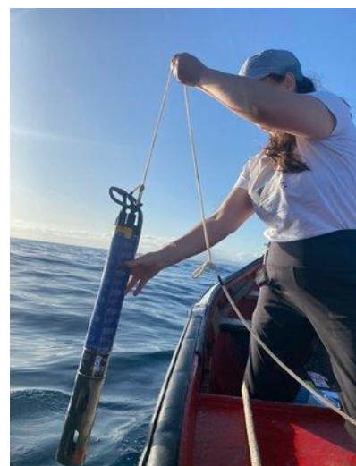
Figure 29: Multiparameter sonde deployment in Santo Antão coast. Source: COAST project
