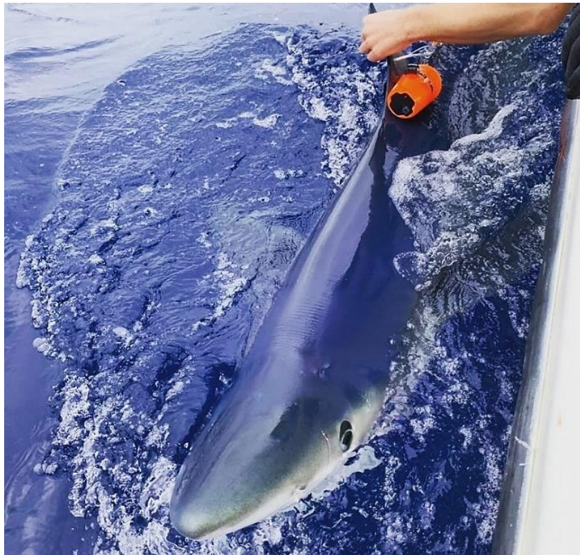
Figure 10: Accelerometer tag orientation on the dorsal fin of a blue shark. Source: Photo credit, Ivo da Costa.
