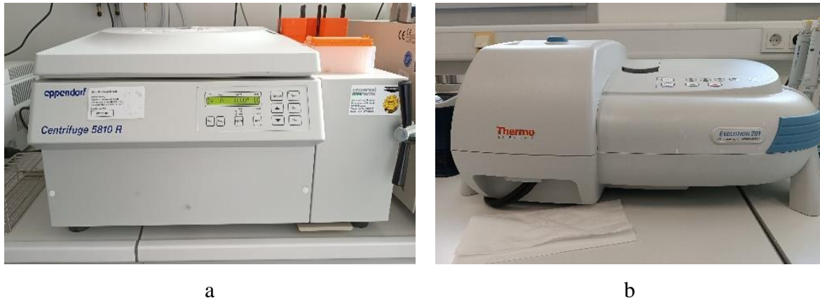
Figure 7: Materials used to analyze the OP sample (Alfred Wegener Institute lab, April 2022). a) the centrifuge and b) the photometer used to measure phosphate in the subsamples.
