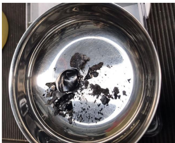
Figure 14 (Metallic-phase and Slag after Hydrogen Plasma Reduction)
