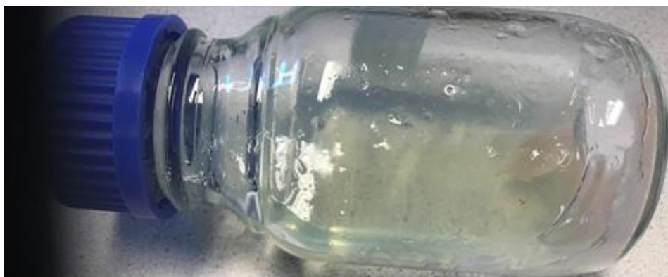
Figure 26: Formation of silica gel after sulfuric acid leaching at 90°C
