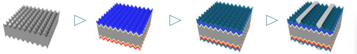
Figure 1-2: Fabrication process of SHJ solar cell at IEK-5
