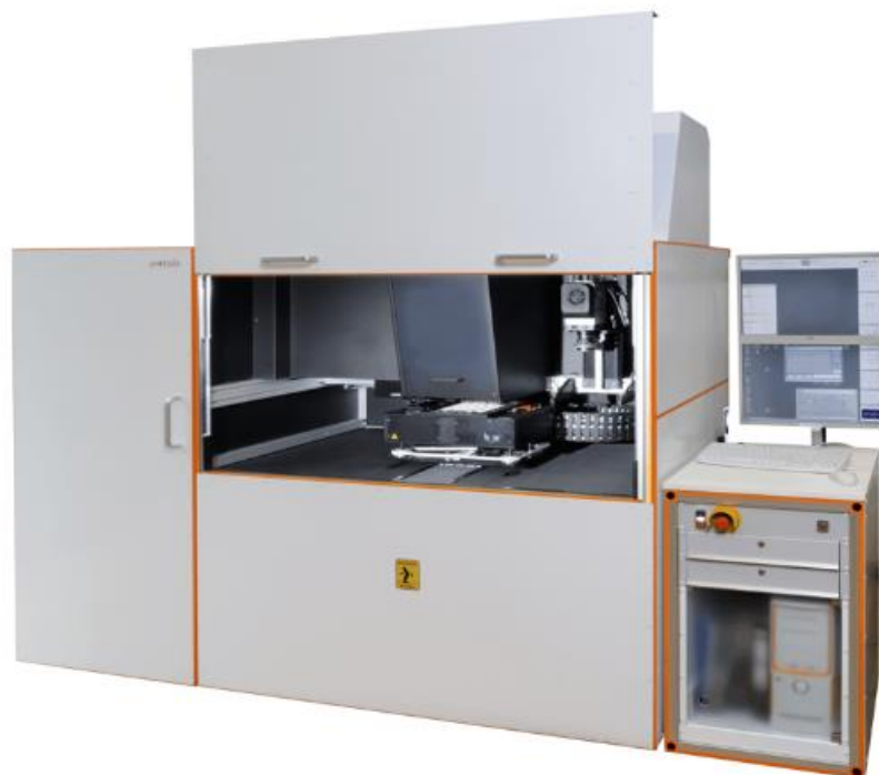
Figure 2-4: LOANA measurement system from pv-tools for characterization of SHJ solar cells performance [53]
