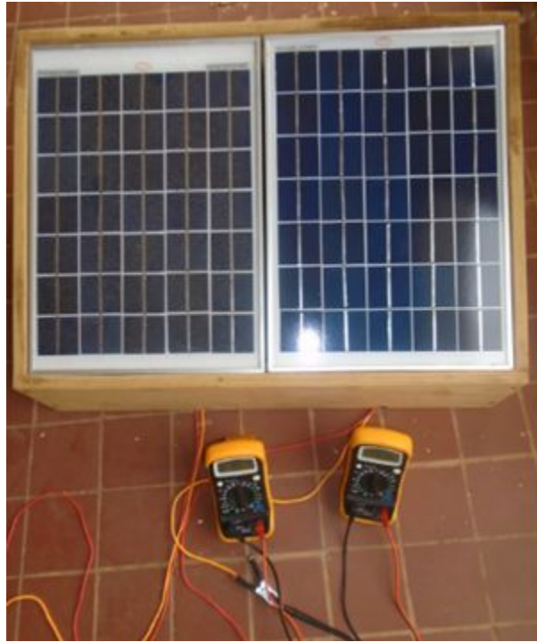
Figure 10. Photos of the PVs during dust experiment with the left one not cleaned during 3 weeks.
