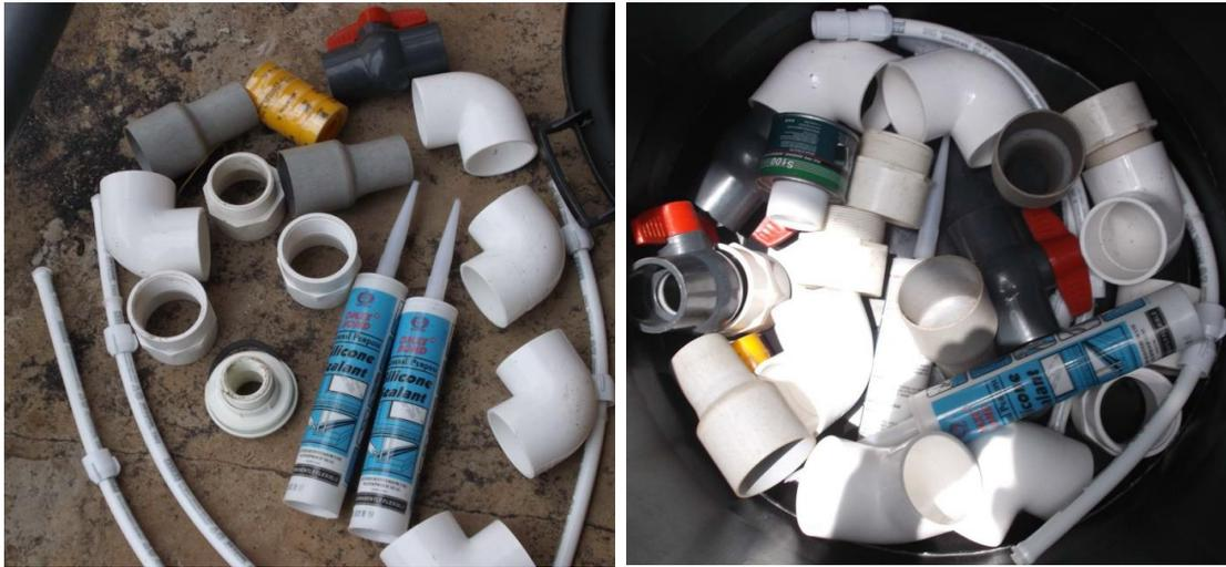
**Figure 2: Some materials used for construction for three 300 liters polytanks as digester and 150 liters tank as a gas holder**
