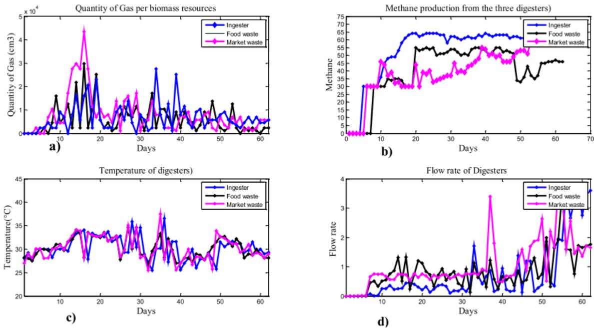
**Figure 8: Biogas production. a) amount of biogas per feedstock through production period; b) methane content per feedstock; c) temperature variation through production period per feedstock; d) flow rate variation through production period per feedstock**
