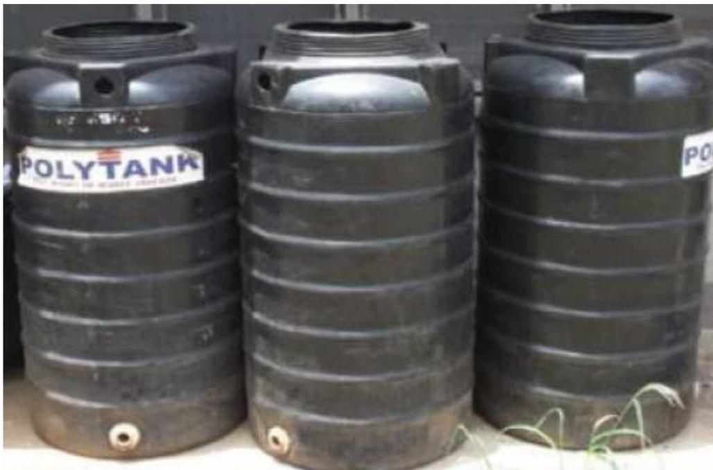
**Figure 3: Polytanks used as a bio-digester**
