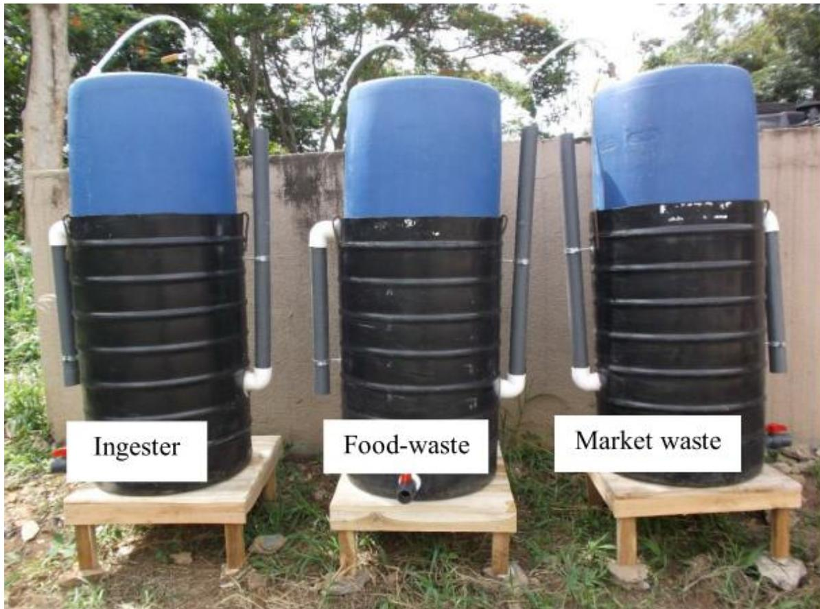
**Figure 5: Three experimental set up for biogas production**
