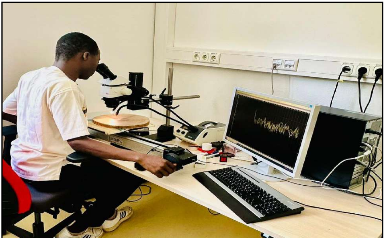
Figure 9: Tree-ring width measurement using LINTAB 6 supported by TSAP software
