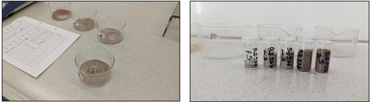
Figure 9: Soil fractions separated, where the left figure shows the dry samples taken out from the oven, and the right figure shows the samples removed from the beakers, weighed and put in small containers.
