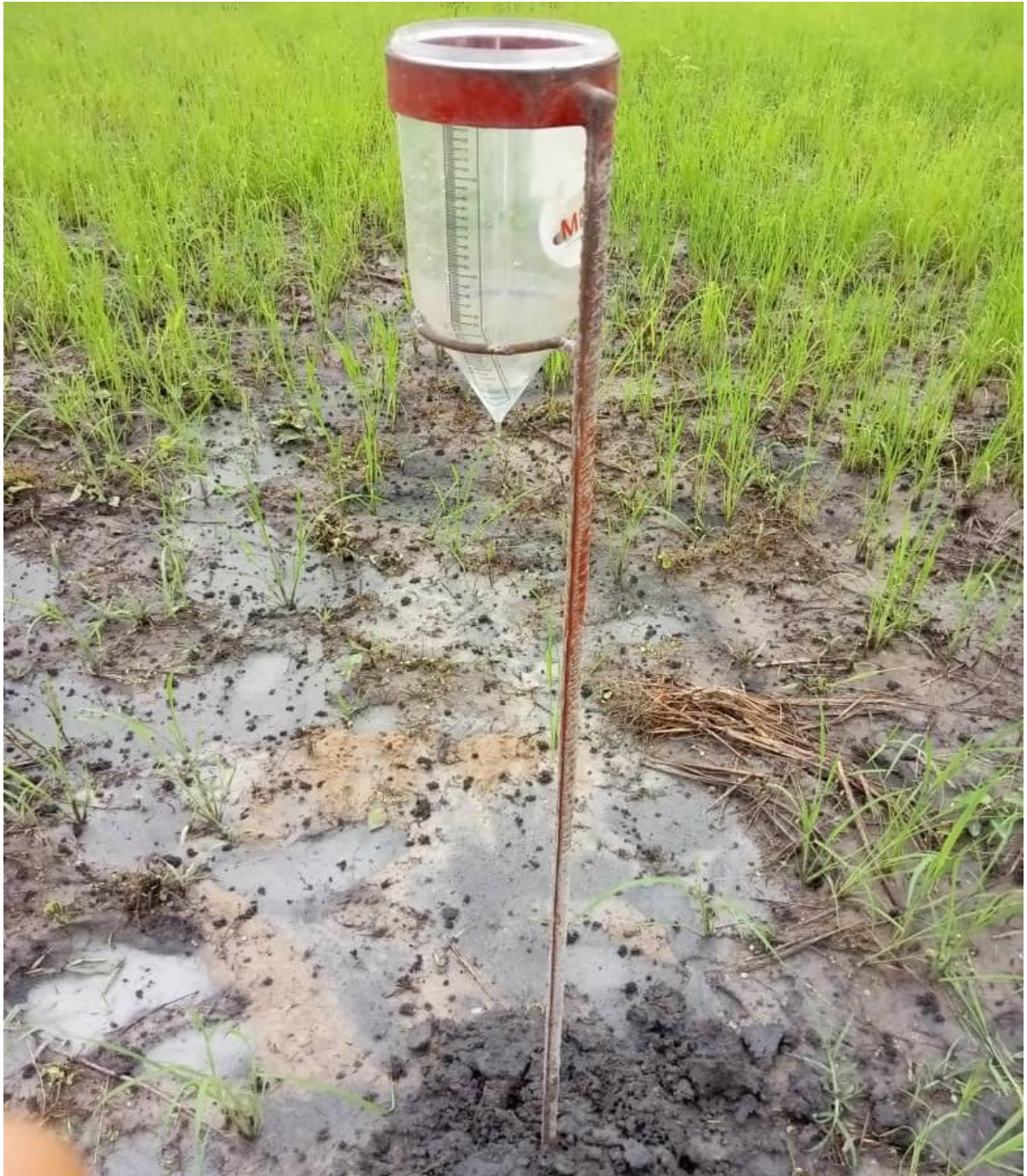
Figure 7. Illustration photo of rainfall gauge installed in the experiment site
