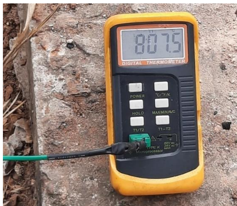
Figure 10: Digital Thermometer displaying the temperature during the pyrolysis process
