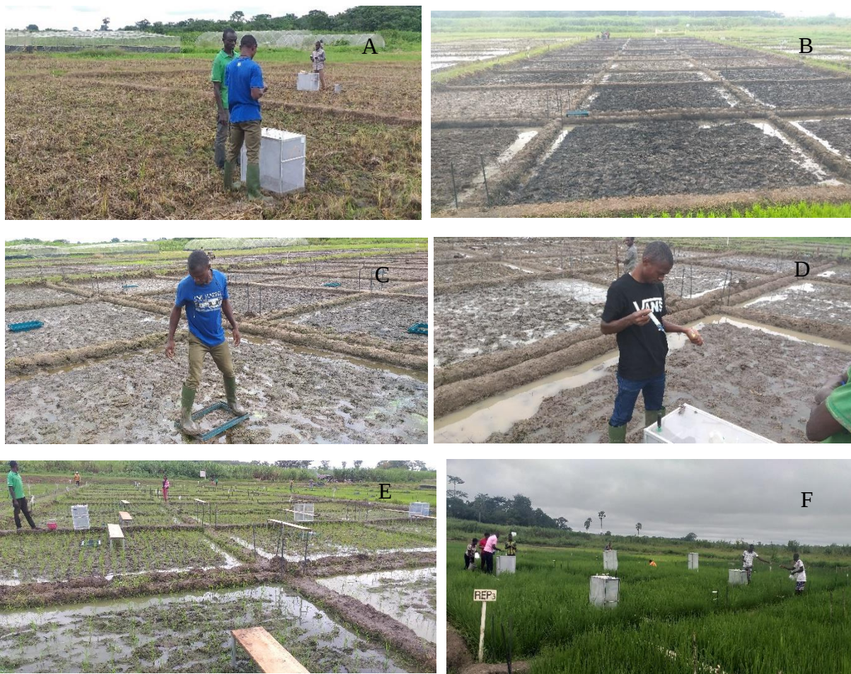
Figure 7: Field gas sampling before treatment application (A), field after treatment application (B), installation of collars (C), gas sampling before rice germination (D), installation of walking board and gas sampling after rice germination (E) and gas sampling at heading stage (F) during the first rice growing season at AfricaRice research station, Mbe, Cote D'ivoire
