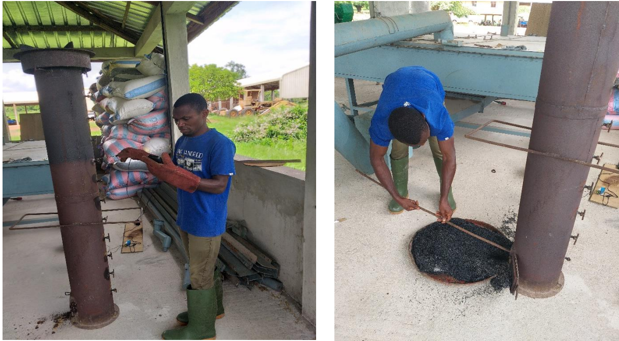
Figure 5: Biochar production for the study of biochar and N-fertilisation effects on GHGs emissions at M'bé, research station Bouaké, Cote d'Ivoire.
