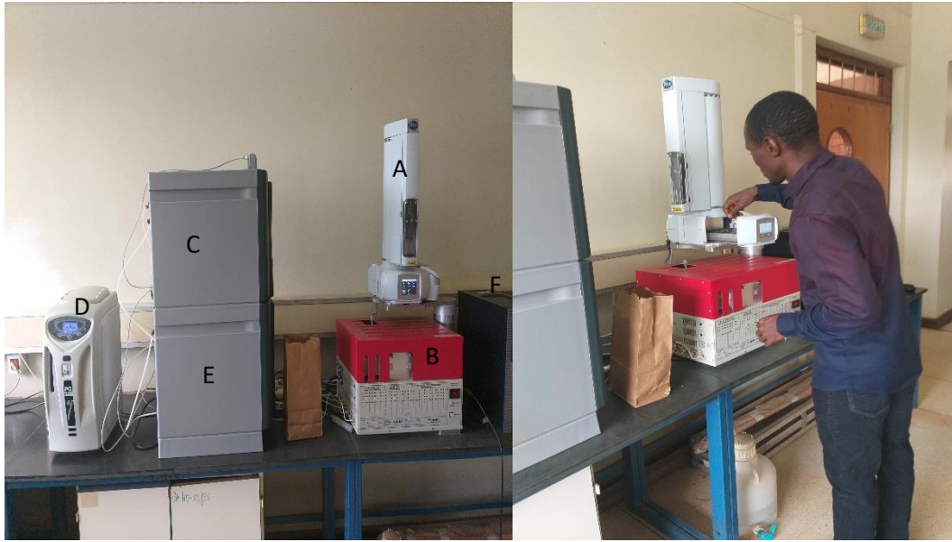
Figure 8: Gas chromatograph system: (A= auto-sampler for taking of gases from vials, B= gas chromatograph equipped with gas detectors, C= nitrogen generator for the detection of N 2 O, D= hydrogen generator for the detection of CH 4 and CO 2 , E= air compressor for generation of pure air, D=visualizing the chromatogram of gases)
