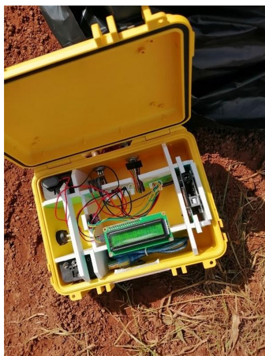
Annex 14: wiring and the complete setup of the developed CO 2 system.
