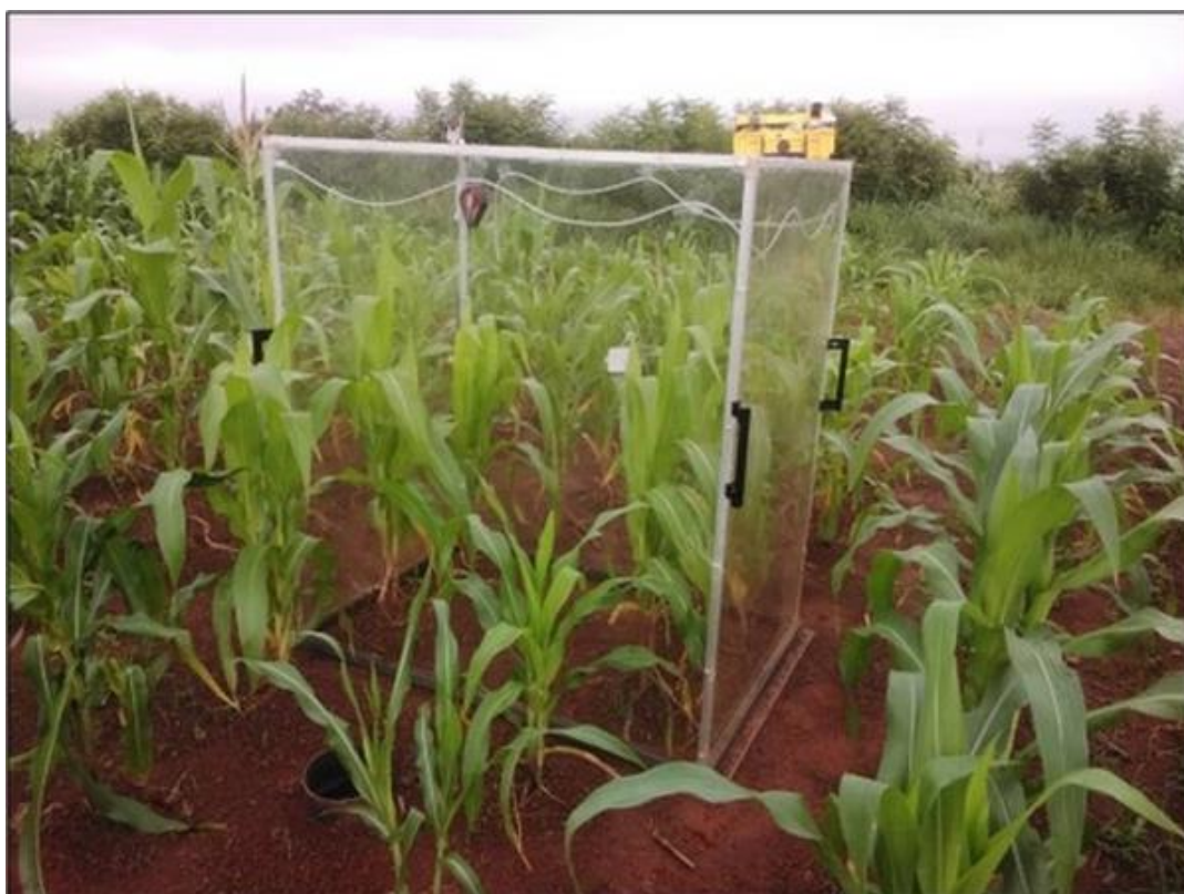
Figure 10: transparent chamber for measuring net ecosystem exchange in Nyankpala Ghana
