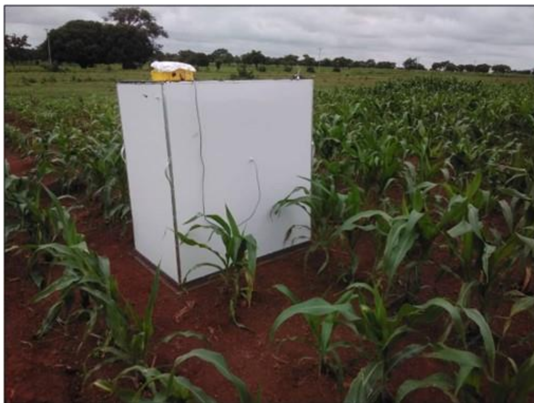
Figure 11: opaque chamber for measuring ecosystem respiration in Nyankpala Ghana
