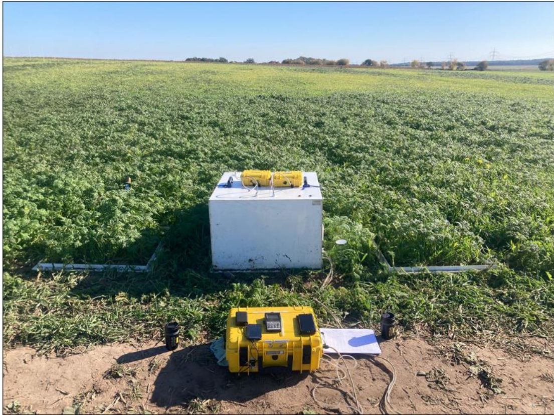
Figure 7: Parallel opaque (Reco) manual closed chamber measurements with a Li-COR 850 IRGA (LI-850, LI-COR, USA) and the developed, low-cost CO 2 and ET flux measurement system at ZALF experimental field near the village of Tempelberg, North-East Germany (52°44'86.2'' N, 14°14'05.1'' E). The developed system was equipped with a K30 FR and SCD30 NDIR, as well as SHT31 and DHT22 sensor.
