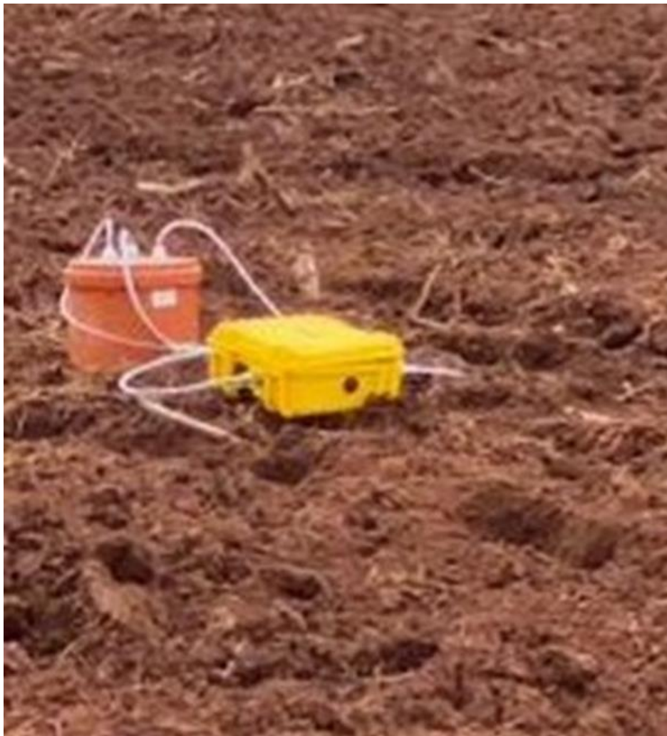
Figure 9: cylindrical chamber connected to the developed CO 2 system for the measurement of heterotrophic respiration after tillage operation in Nyankpala experimental field.
