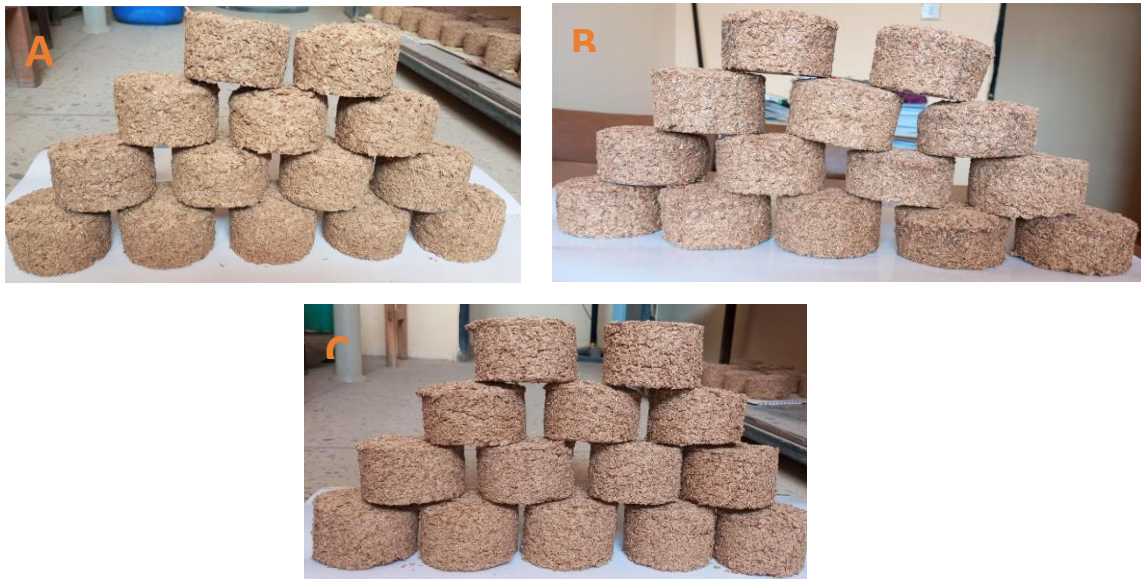
Figure 2. Briquettes produced with rice husk and (a) Locust bean pulp (LBP) binder, (b) Sweet potato peel (PPL) binder, (c) Cassava starch (CSS) binder
