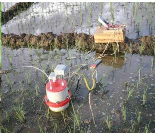
Plate 7: Soil CO 2 flux monitoring under rice
