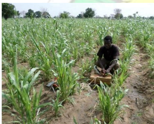
Plate 8: Soil CO 2 flux monitoring under sorghum
