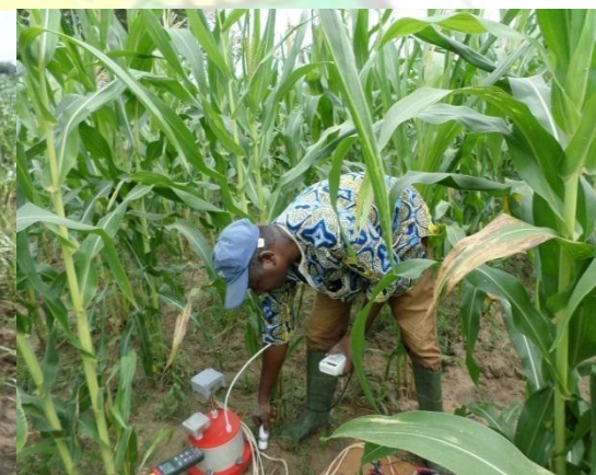
Plate 9: Soil moisture measurement using Delta T device
