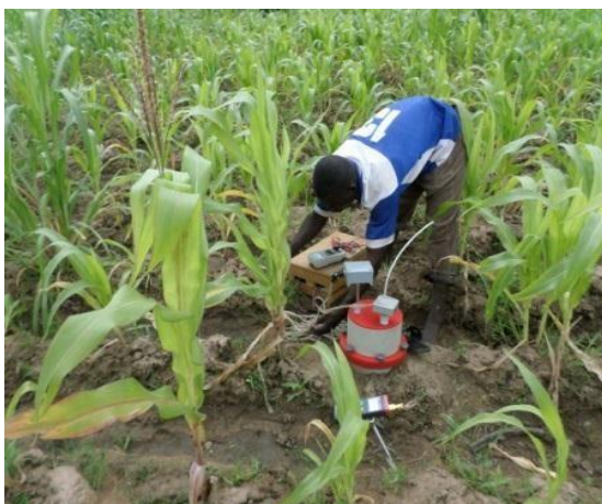
Plate 6: Soil CO 2 flux monitoring under maize
