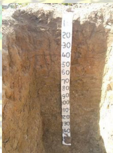
Plate 2: Calcic Gleysol (WRB/FAO 2014) soil profile
