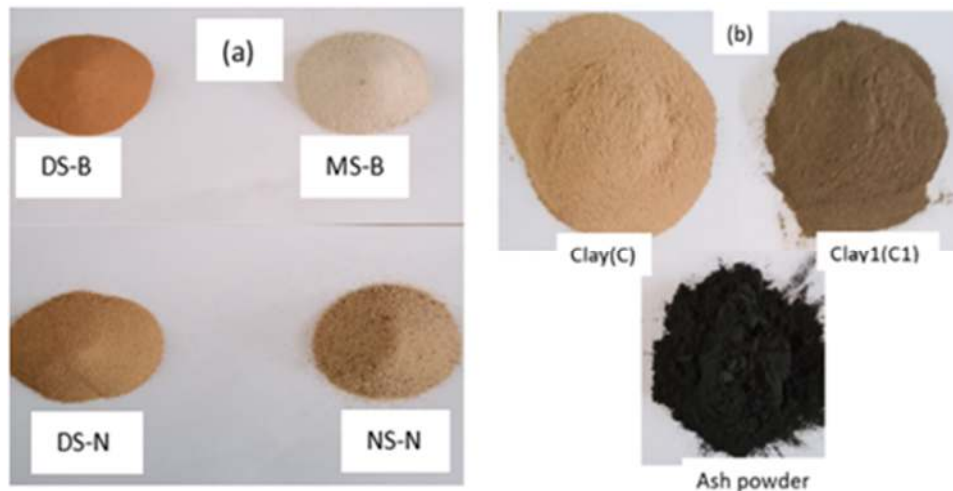
Figure. 2. 4. Raw materials: (a)-Dune sand from Burkina (DS-B) and Dune sand (DS-N) from Niger, mining sand from Burkina (MS-N), Natural sand from Niger (NS-N); (b)-clay (C) from Malgsombo, Clay (C1) from Tchériba and coal bottom ash from Agadez.
