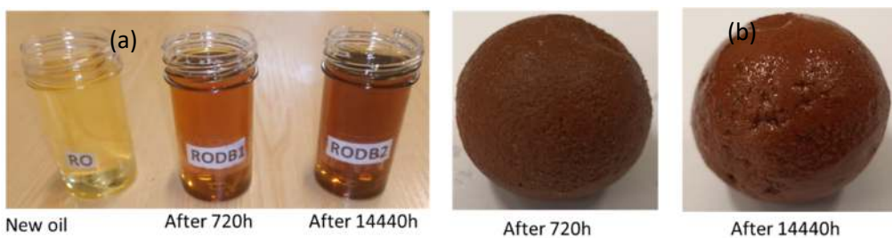
Figure. 3. 17. Aspect of JCRO (a) and ceramic balls (c) before or after heat treatment.
