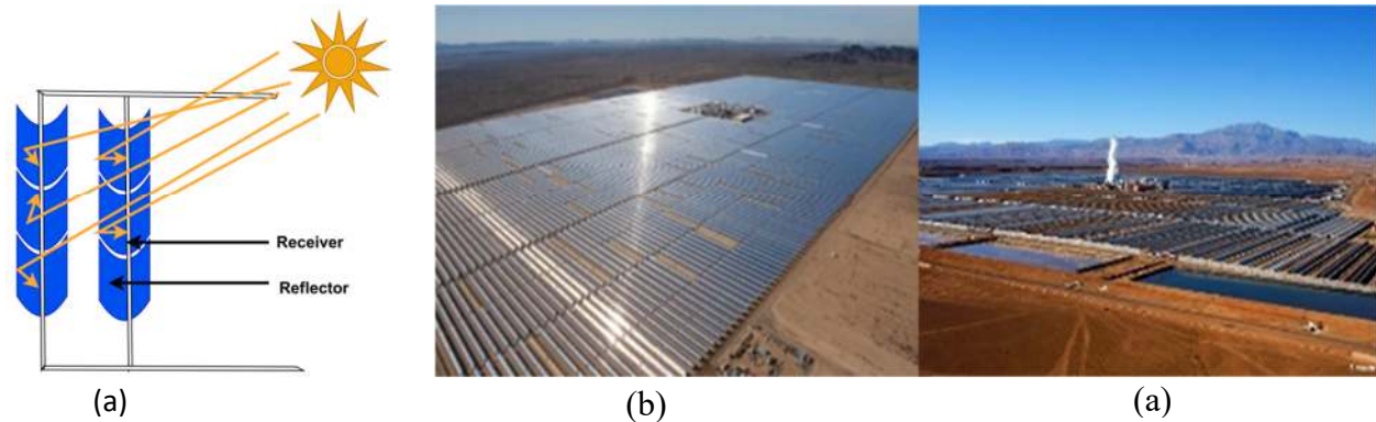
Figure. 1. 4. Parabolic trough collector (a), Solana power plant [27](b), Noor Ouarzazate I power plant [12] (c).
