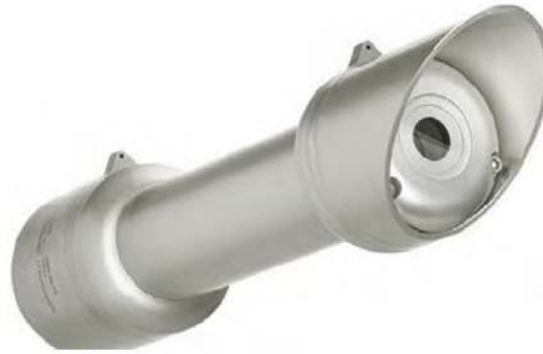
Figure. 5. 5. DR15-A1 C/ass 8 pyrliometer: the externa/ housing [222]
