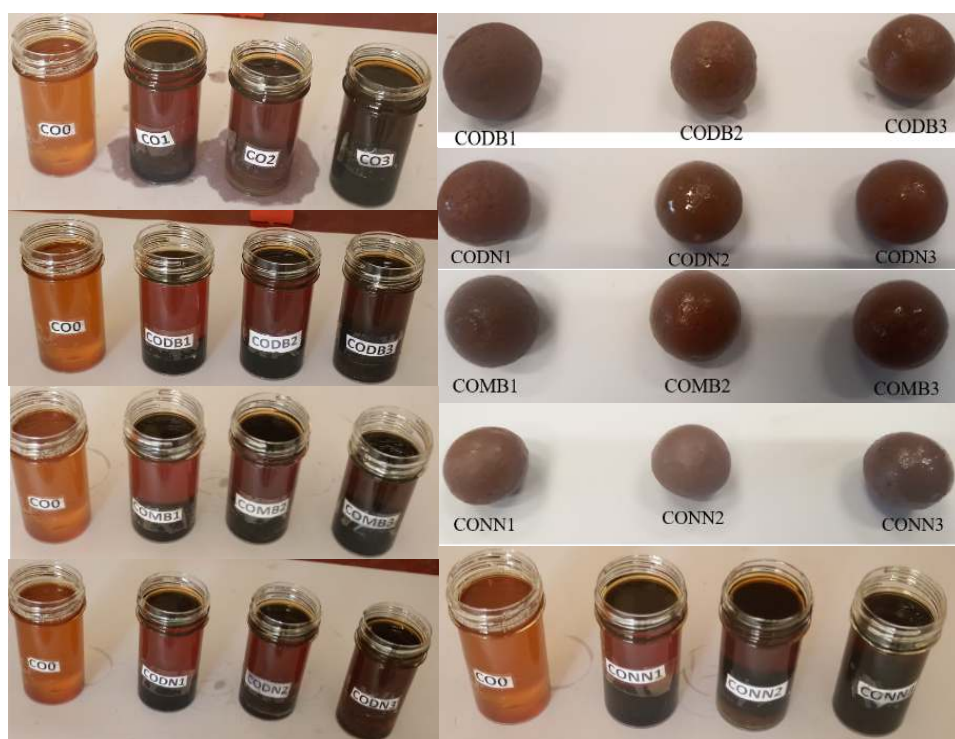
Figure. 3. 7. Oil and ceramic balls before or after heat treatment. Co is crude oil, the number 0, 1, 2, 3 indicate the reference oil and the oil after the first, second and third month. The same labelling
