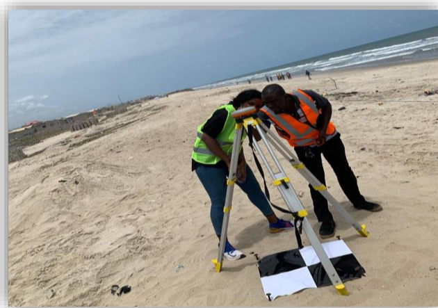
Plate 3.2: Measuring the geographic location of Ground Control Point (GCP) Source: Author (2023)
