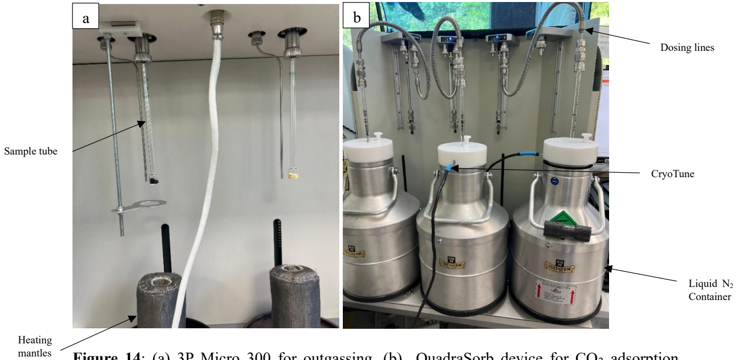
Figure 14: (a) 3P Micro 300 for outgassing, (b) QuadraSorb device for CO 2 adsorption isotherms
