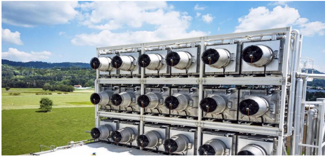
Figure 4: Direct Air Capture (DAC) Device. ( SOLARIFY , n.d., 2025)
