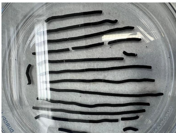
Figure 9: Strands of PAN-DMF mixture extruded for pelletization
