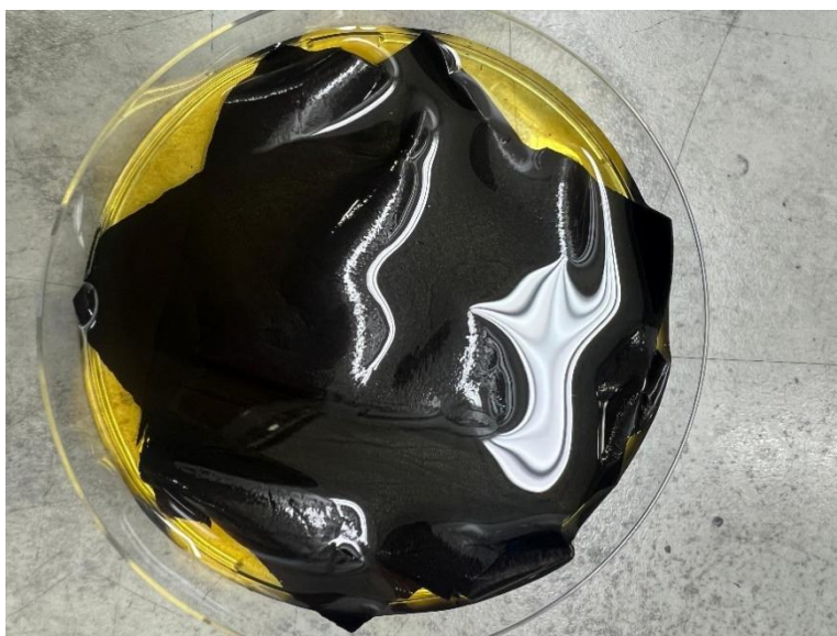
Figure 12: PAN-stabilized fibers soaked in KOH solution
