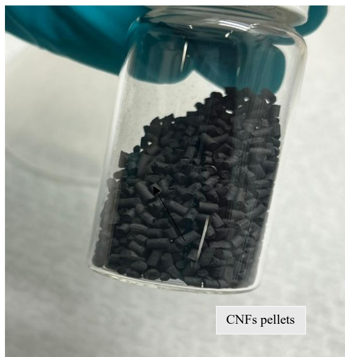
Figure 10: Carbon nanofibers after carbonization.
