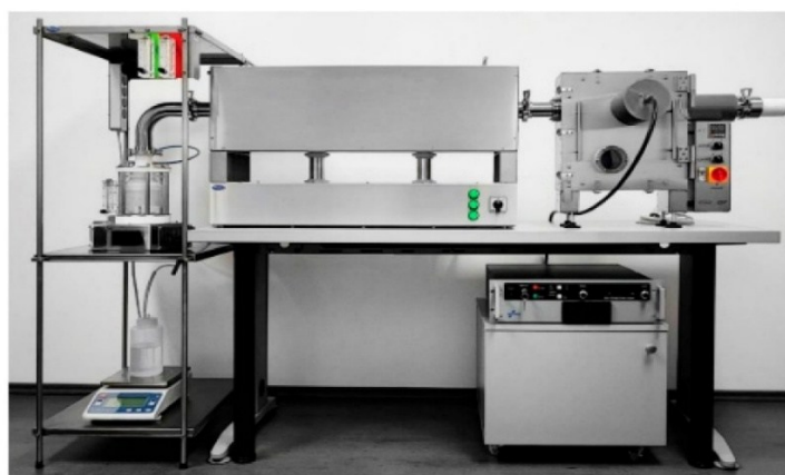
Figure 8: An advanced setup of the ultrasonic spray pyrolysis (USP) device
