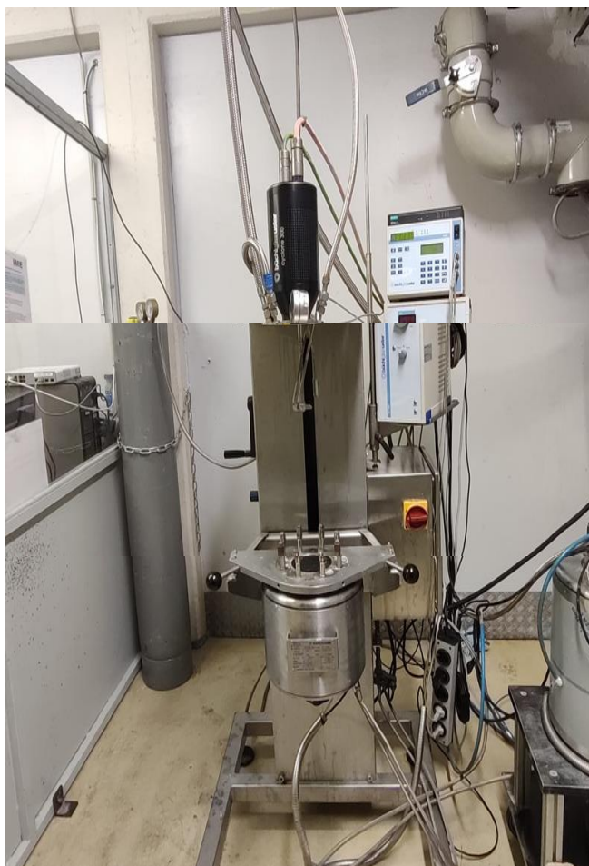
Figure 11:: Experimental Setup of Leaching and Schematic Diagram of Autoclave (Stopic & Kostic, 2024)
