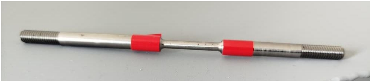
Figure 0.14: The test sample with the non-reactive insulating tapes
