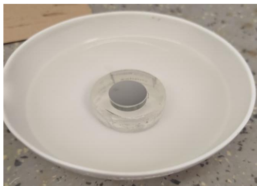
Figure 0.13: Etching procedure inside the solution
