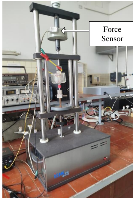
Figure 0.18: Complete in-situ SSRT setup
