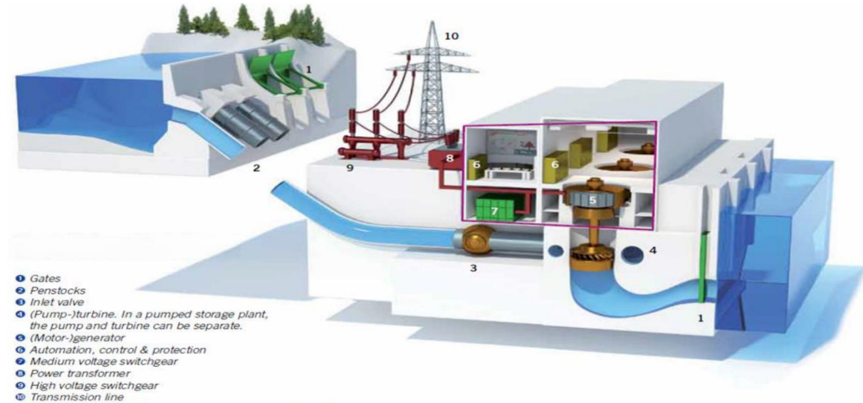
Figure 2: Layout of Reservoir-Storage Hydropower Plant. Source: (European Commission, Joint Research Centre, Quaranta, E., Georgakaki, A., Letout, S., Mountraki, A., Ince, E. and Gea Bermudez, J., 2024)
