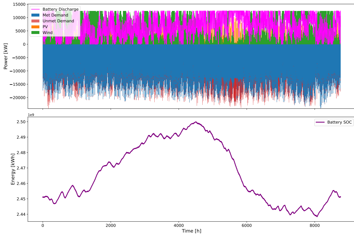
Figure 4.3: Hourly energy generation and demand balance (top), and battery state of charge (bottom) over the simulation year for Scenario 2
