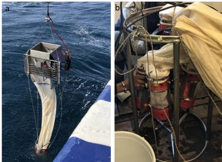
Figure 5: Multinet Type MIDI. a showed the Multinet going in the water, b showed the assembly of the 5 Nets
