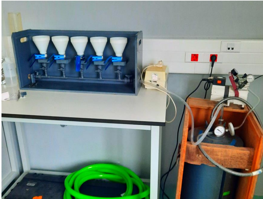
Figure 2: Seawater samples filtration apparatus at the Ocean Science Centre in Mindelo.
