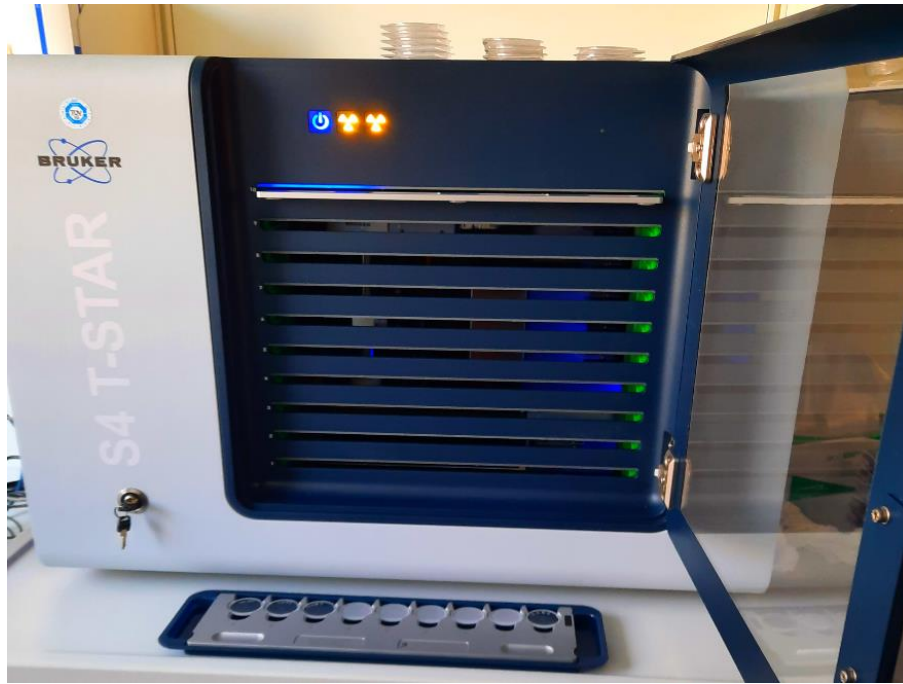
Figure 10. The S4 T-STAR spectrometer used for the metals analysis shows the ten trays' entries and one tray on which nine carries are placed
