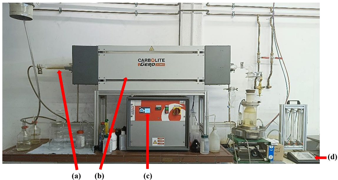
Figure 2.5. Carbolite setup for USP-HR technique with some specific features (a) alumina tube, (b) large furnace, (c) furnace control panel, (d) automatic ultrasonic generator
