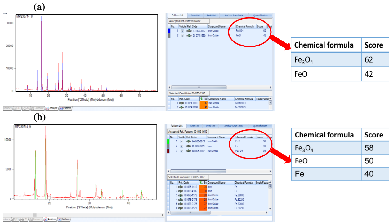
Figure 3.4. XRD patterns of Fe 2 O 3 particles produced at (a) 700 °C, (b) 950 °C
