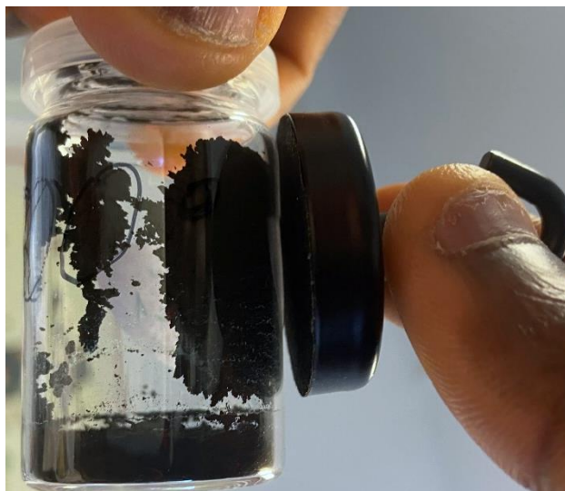
Figure 3.17. AgCoCuFeNi samples with magnetic properties
