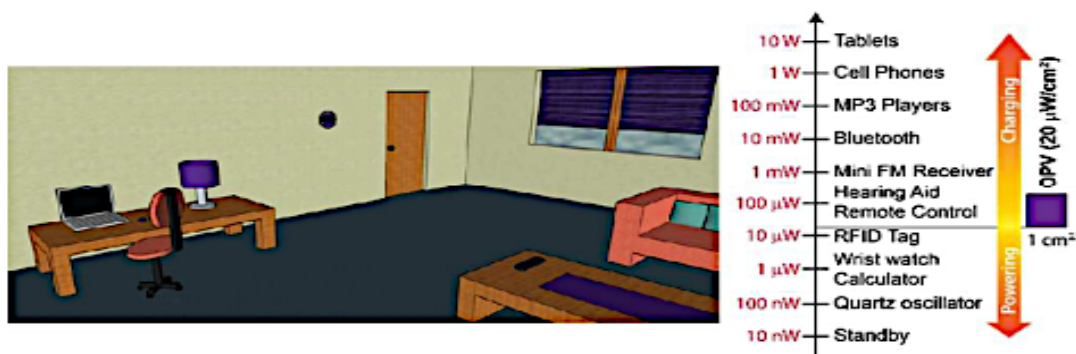
Figure 1.1: Indoors Photovoltaic application (left) a future house with OPV thermostat, computer mouse, remote control, curtains, lampshades and coffee table mats for re-using indoor light; and (right) power requirements for various devices used indoors and power from a 1 cm 2 OPV cell (L. Cutting, et al., 2016).
