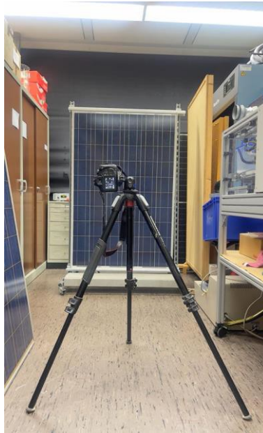
Figure 4: Real Setup of The Electroluminescence Measurement.
