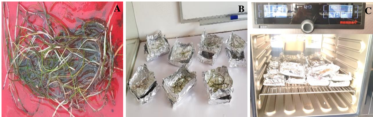
Figure 5: showing photographs of seagrass biomass data collection procedures in the Laboratory: seagrass core sample(A); separated above and below ground biomass in the pre-weighed aluminum foil tins(B); Drying separated below and above ground biomass(C).
