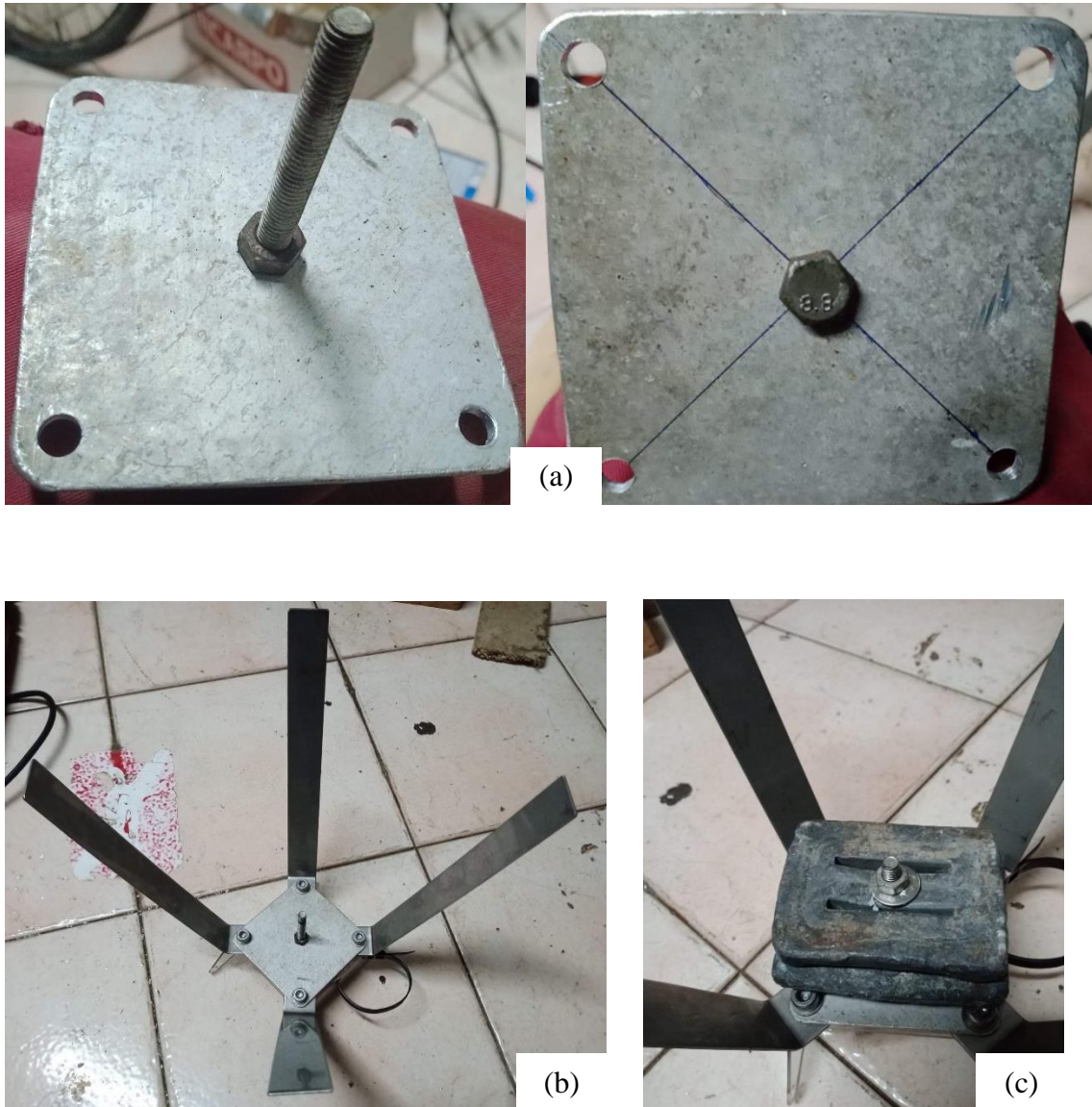
Figure 24: Standing frame modified: (a) Square heavy metal; (b) Square heavy metal fix at the bottom of the standing frame; (c) Weights attached to the support square heavy metal on the standing frame.
