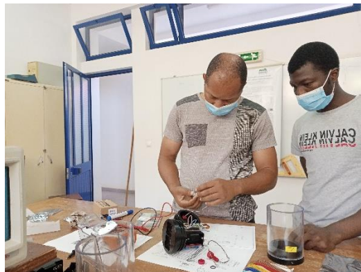
Plugging of the Temperature sensor to the I2C bus splitter
