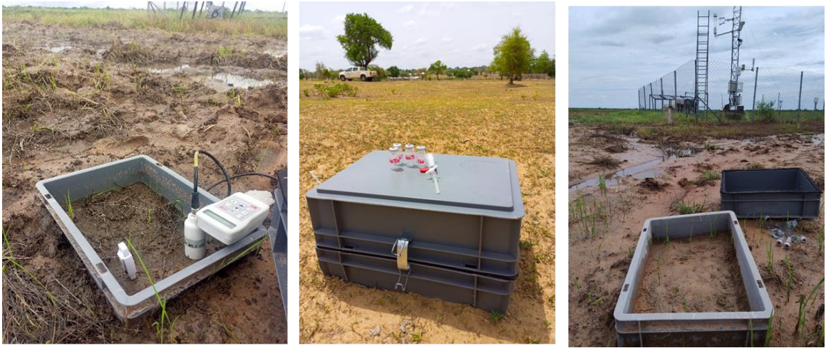
Figure 3.8: Chamber-based greenhouse gas sampling plots; closed (middle) and opened for soil moisture and temperature measurements (left and right) in a rice field at Janga, Upper-East Ghana
